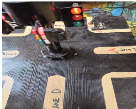
Fig. 16: Lane D is showing red (L.E.D.), which is stop vehicles
