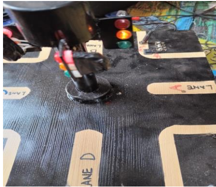
Fig. 15: Lane D is displaying Ready to Stop, which is a yellow light-emitting diode
