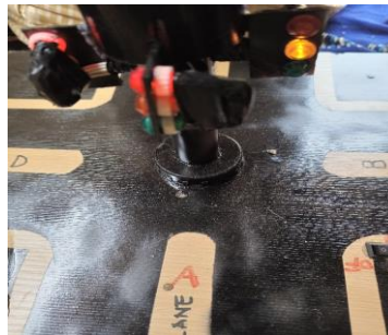
Fig. 7: Lane A is showing ready to stop, which is yellow (L.E.D.).
